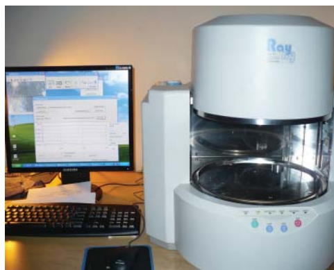
Fig. 2: EDXRF analysis determines the chemical composition of a gemstone, aiding in narrowing down the possible origin of a gemstone. Photo: Lore Kiefert, ©AGTA GTC
