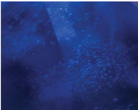
Figure 3B: Sapphires from Madagascar can look very similar to Kashmir sapphires. However, a closer look shows that the pattern in Madagascar sapphire is more regular than in Kashmir sapphire. Photo: Hpone-Phyo Kan-Nyunt, ©AGTA GTC
